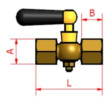
Body made from unpolished brass; handle hard black plastic. Used where isolation of the pressure gauge is required.
